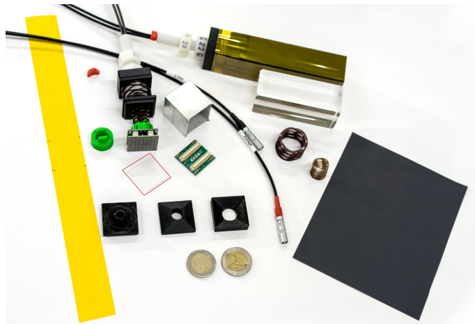
Figure 9: LYSO-SiPM module before and after assembly. Module ingredients are also shown. With the red square, the silicon interface is exposed.
